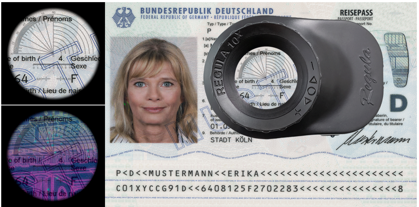
Regula 1004MU on a passport page - LED light sources: oblique white, ultraviolet 365 nm - 10x magnification
