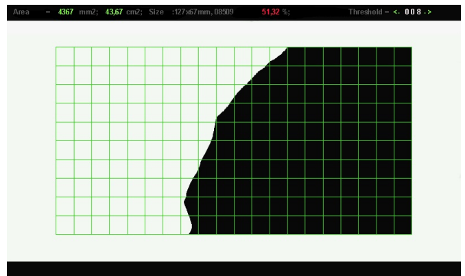
Automatic measurement of the banknote area (residual area)
