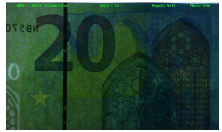
Fragment of the examined banknote in white transmitted light. 2x magnification on the monitor
