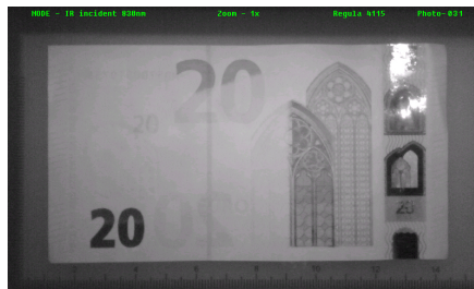
Comparison between the examined banknote in infrared incident light (830 nm) with the reference banknote from the database
