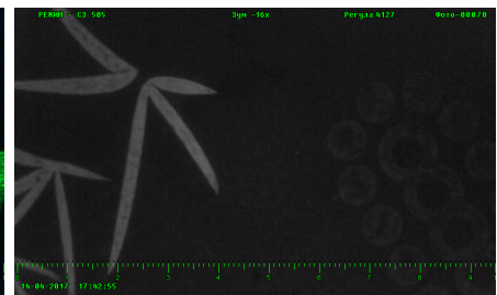
Fragment of the examined banknote in cyan high-intensity incident light (505 nm). 16x magnification on the monitor
