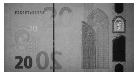
Transmitted infrared (870 nm) light
